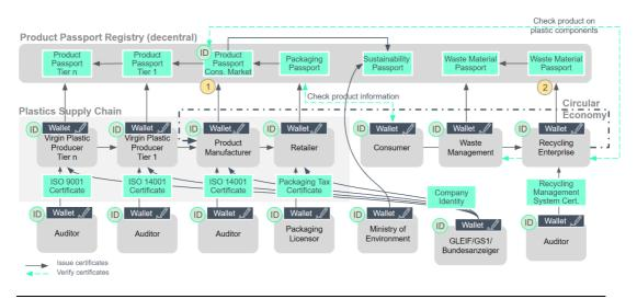
Figure 3: Functional Architecture: Physical Objects Flow and Data Flow with W3C Decentralised Identifiers and W3C Verifiable Credentials (digital Product Passport) for a Circular Plastics Economy. Own representation.
