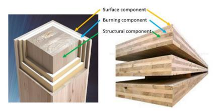
Figure 3-7: Examples of new wood materials in Japan
