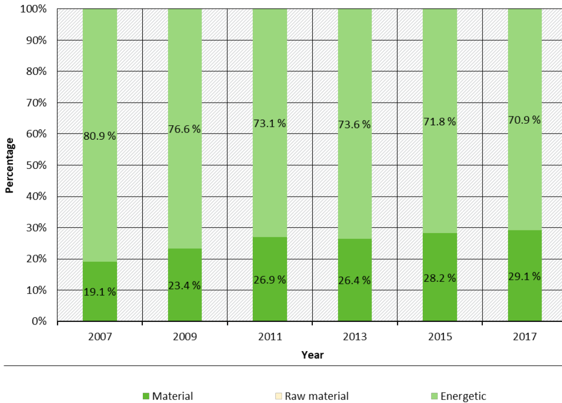
Figure 20. Proportional development of recycling types used for plastic waste from the construction sector in the period from 2007 to 2017.
